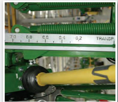
The McHale R 62-72 & R 68-78 twin-rotor centre delivery rakes offer a number of different working widths as illustrated in the table above. The variable working width is adjusted hydraulically from the tractor seat.
