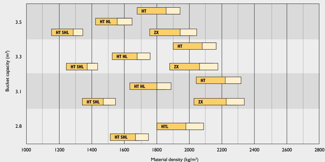
HT = Standard height arm HL = High lift arm SHL = Super high lift arm ZX = Z bar
