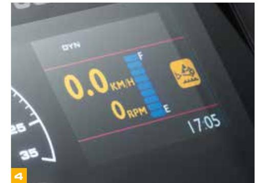
A new auto engine shutdown feature saves fuel by switching off the engine when the machine is left idling. Idle time can be set by the operator from the cab seat.
